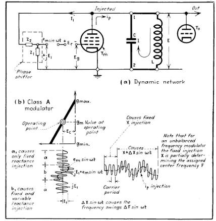
Fig. 3.—Dynamic network of oscillator tube and reactance tube injector circuit (α), with wave forms of modulated and unmodulated signals illustrating variation of transconductance of modulator tube
