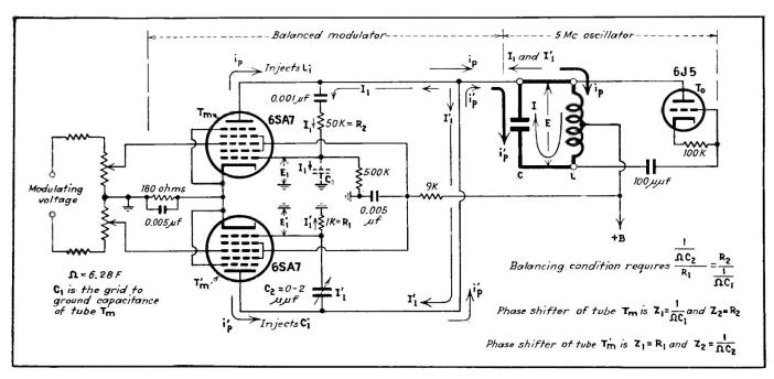
Fig. 4—Diagram of balanced modulator and oscillator tube to illustrate the current and voltage conditions which occur for a balanced modulator
