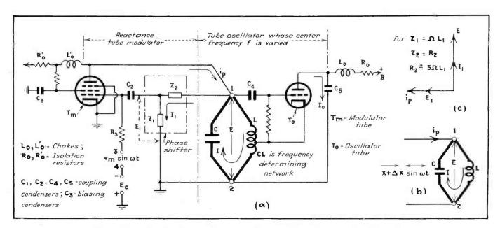
Fig. 1—Schematic wiring diagram of reactance tube modulator and associated oscillator tube. The assigned carrier frequency is  ${\bf f}=\Omega/6.28$ ; the modulating frequency is  ${\bf f}=\omega/6.28$
