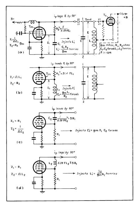
Fig. 2—Schematic wiring diagram of four types of reactance tube networks, with their design equations
